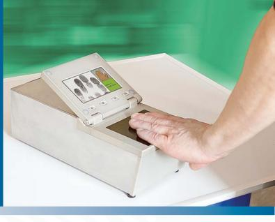
The **DS-30NM** is a forensic quality fingerprint scanner manufactured as a separate optical unit driven by a backbone computer (including a notebook).
