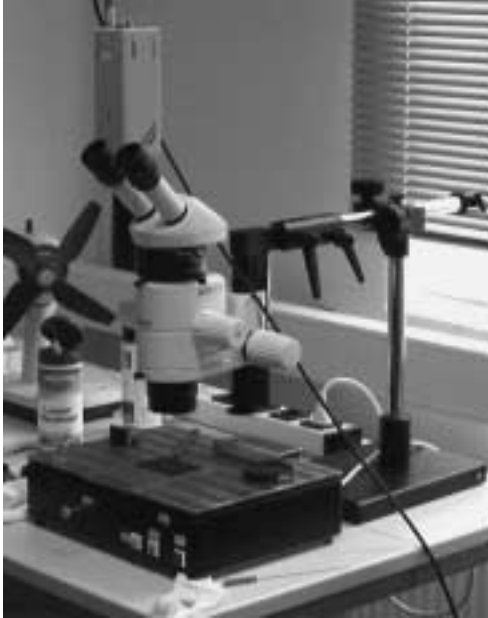
Plate 8 "MOA-KOF" device with Leica microscope and Kappa camera, general view.
